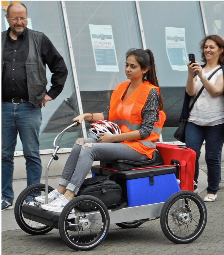
Fig. 10 Seat position, weight distribution and joystick steering
