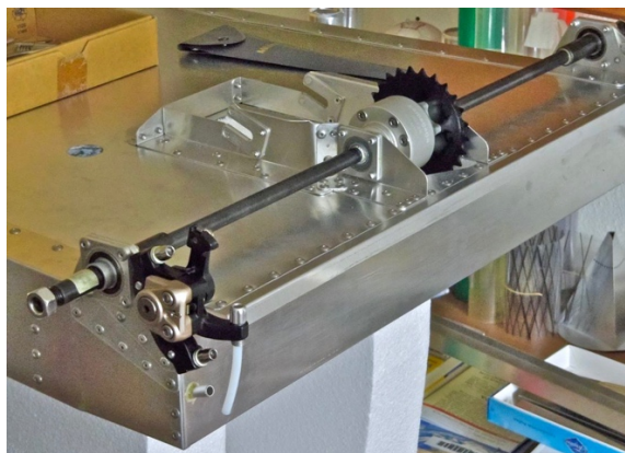
Fig. 8 Half-axles of rear wheels with differential Fig. 9 Final assembly with drive train and controller
