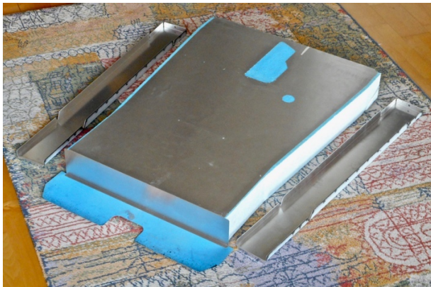
Fig. 5 Platform sandwich and side walls
