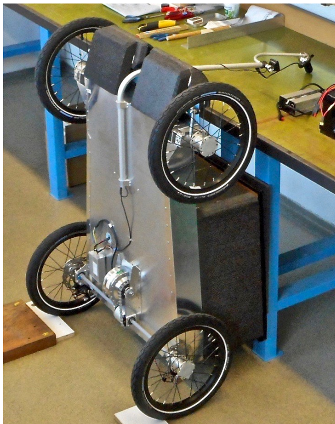
Fig. 8 Half-axles of rear wheels with differential Fig. 9 Final assembly with drive train and controller
