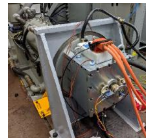
Overall WFSM rotor with brushes and slip rings mounted on dynamometer
