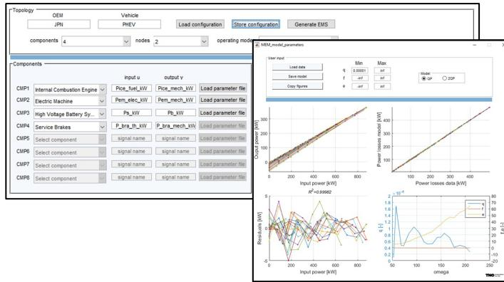
Convex control model calibration & supervisory optimal control algorithm generation tool
