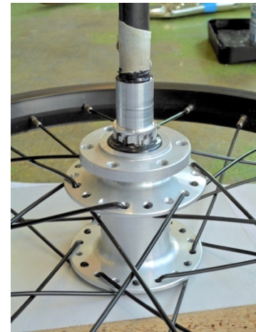
Fig. 14 Permanent connection between half axle and hub of the rear wheel by adhesive bonding
