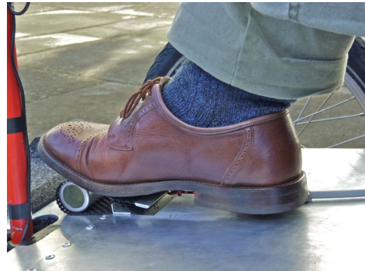
Fig. 12 Foot brake with cables for the two mechanical disk brakes on the rear wheels, with a rolling belt
