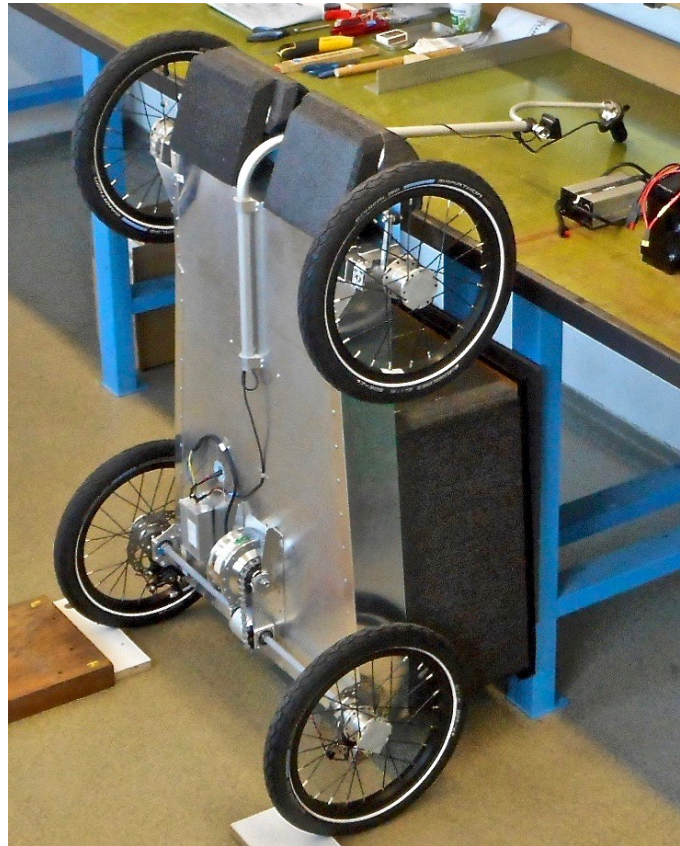
Fig. 8 Half-axles of rear wheels with differential Fig. 9 Final assembly with drive train and controller
