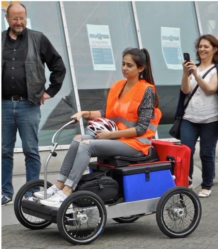
Fig. 10 Seat position, weight distribution and joystick steering
