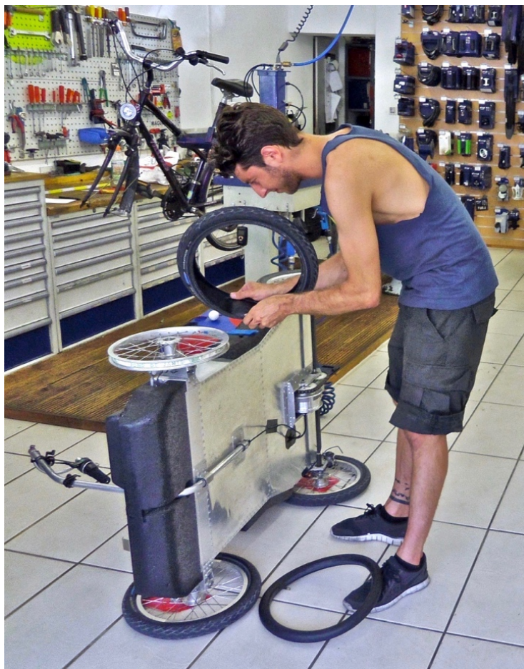
Fig. 15 Repair of a flat tire without removing the wheel
