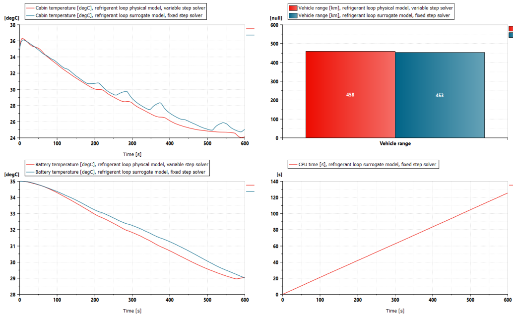
Figure 14: Comparison between physics-based and fixed step solver model and CPU time of the fixed step model
