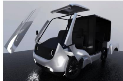
Figure 7 Modular e-quad design
