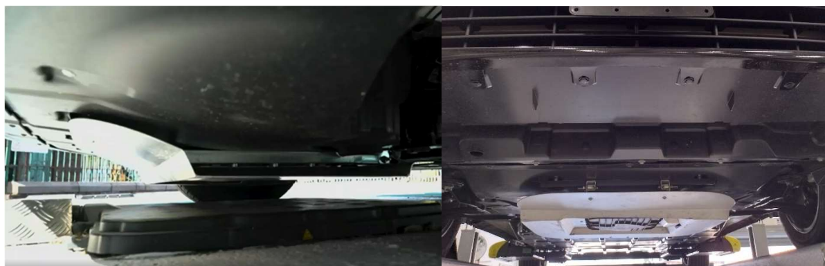
Figure 6: Photos from the private pilot showing side and front views of VA and EM shield mounted using a front position on the vehicle, with limited ground clearance.
