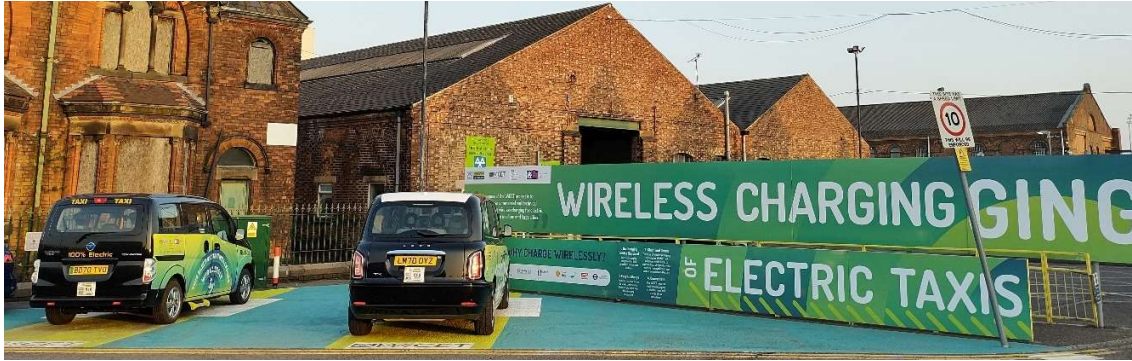
Figure 2: WPT installed at the Nottingham Eastcroft private pilot site
