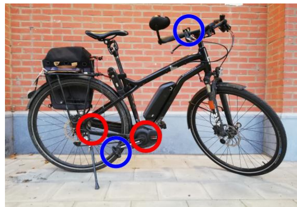
Figure 2: Schematic of the speed pedelec measurement module and auxiliary measurements using a Garmin Edge 510 and the Assioma duo power meter.
